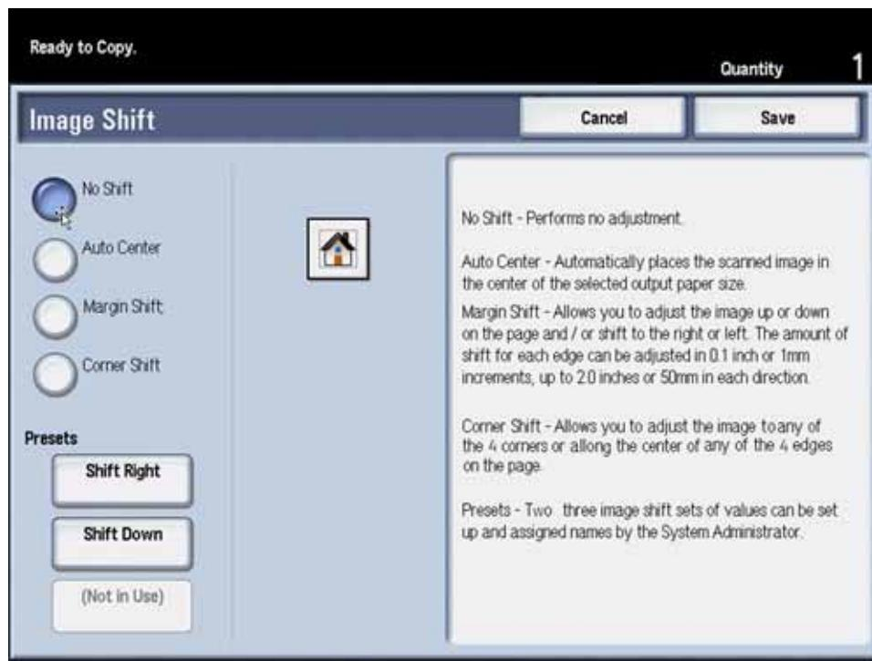
The **No Shift** option is the machine default setting for the Image Shift feature.
